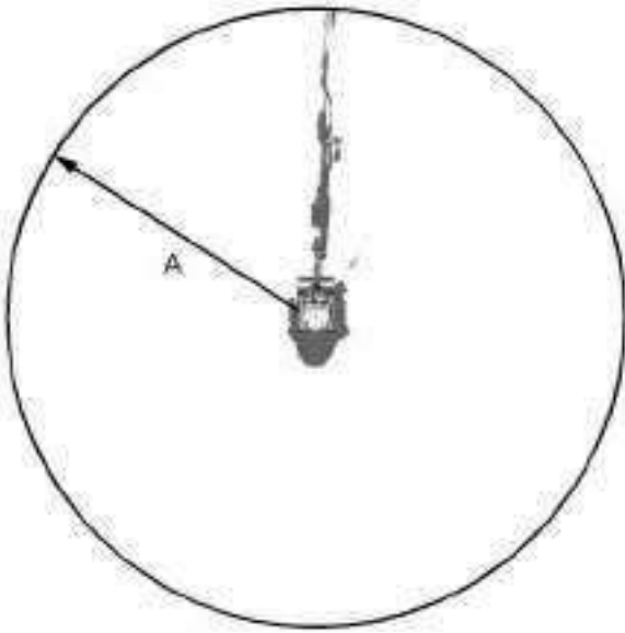
Illustration 54 g06321906 Top view of the machine, ground level visibility, with available left side mirror and right side mirror (A) 12 m (39 ft)
